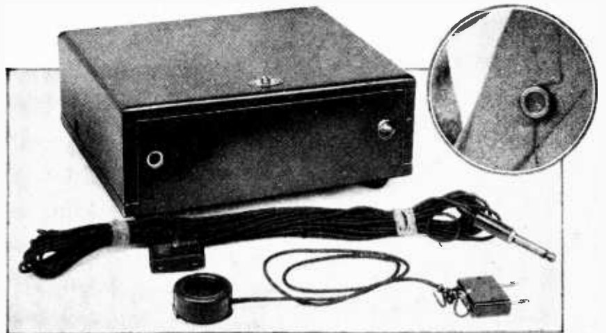
FOR RESTLESS ANNOUNCERS. Here, fresh from America, is a lapel microphone outfit, developed by the Bell Telephone Laboratories, which permits an announcer or public speaker to "ramp around the platform" while broadcasting.
