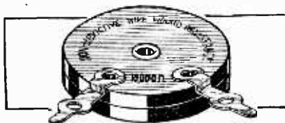
The new disc-type non-inductive resistance made by British Electric Resistance Co., Ltd. The resistance is of spirally wound fine wire.
