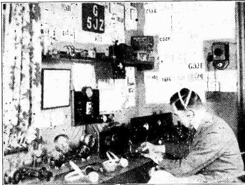
AN EFFICIENT LOW-POWER STATION. G5JZ, owned by Mr. C. W. K. Sands at Heathfield, Sussex, has worked all Europe and parts of Africa with an input of 7 watts on the 7 megacycle waveband. In the foreground is seen the 80-metre set, then the 20-metre receiver and the 40-metre crystal-controlled transmitter, while the amplifier is partly hidden behind the operator.
