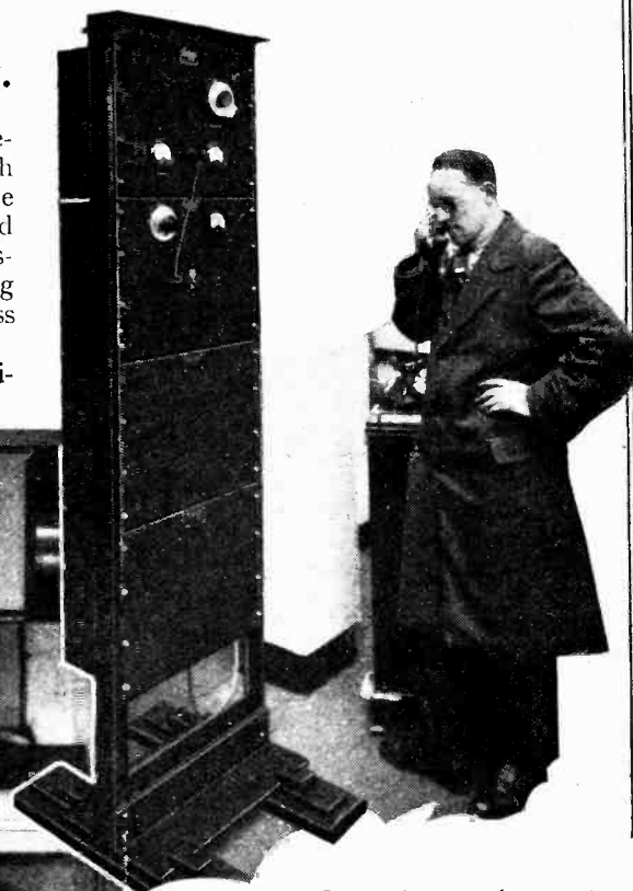
Conversing on the 2-metre transmitter. The lowest picture shows the super-regenerative receiver used in the demonstrations. Note the short vertical aerial.
